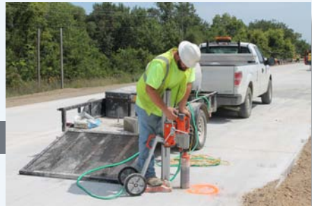
Adam Brooks drilling a concrete sample to be tested on Route 24
