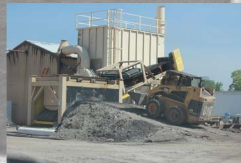
Ideker's fine grind system produces more effective liquid AC to coat the aggregates.
